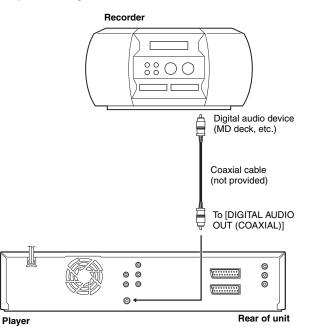
Connect the unit and a digital audio device using an optional coaxial cable.
